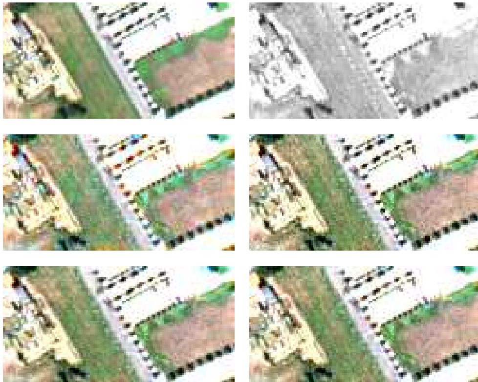
Fig. 9. ROSIS dataset: (Top left) Reference. (Top right) PAN Image. (Middle left) Adaptive IHS [63]. (Middle right) MAP [25]. (Bottom left) Wavelet MAP [26]. (Bottom right) Hamiltonian MCMC.
